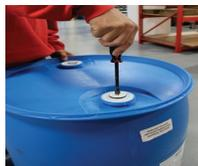
A large flat blade or #4 Phillips screwdriver may be used to remove shipping plug.
