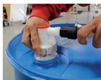
Turn Coupler Lock Ring clockwise fully until stop is reached to connect and open.
