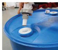
Vent port on the coupler may either be left open to vent to atmosphere or be outfitted with a check valve to allow make-up air into the drum.
